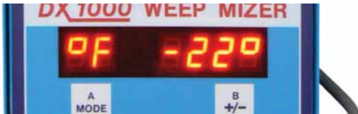
If your Weepmizer is reading -22 that indicates that it is not seeing a sensor
